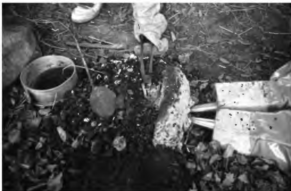
Fig. 4: An open bowl shaped forge furnace was dug some 25 CMS wide and 6 CMS deep, with a tuyere of clay at one side containing the central blow hole for the bellows. Once the furnace was heated, peat charcoal was introduced and we started working on a lump of iron made in Jutland during an experiment with wood charcoal. (DM-fig4.tif)
