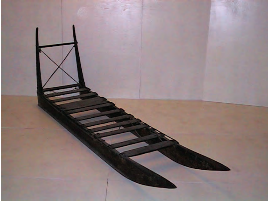
Fig. 1. "The dead man's sled" which Ludvig Mylius-Erichsen obtained from Kolotengva / Kulutenguaq/ Qolugtinguaq, and donated to the Ethnographic Museum in Oslo. The sled is probably built from driftwood . Every joint is lashed with leather thongs. Only the runners are iron. In the old days, runners were made from bone or ivory. Photo: Eivind Bratlie, Museum of Cultural History. Oslo
