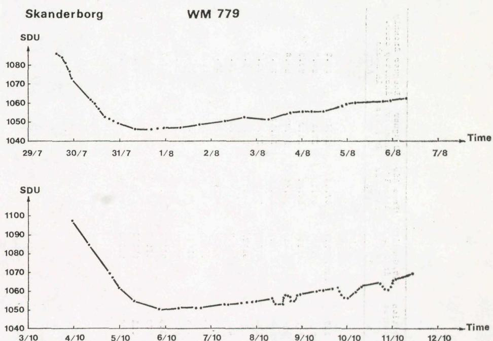
Fig. 7. Drift curve for Worden Master gravimeter No. 779 at station Skanderborg during connection and disconnection of the battery.
