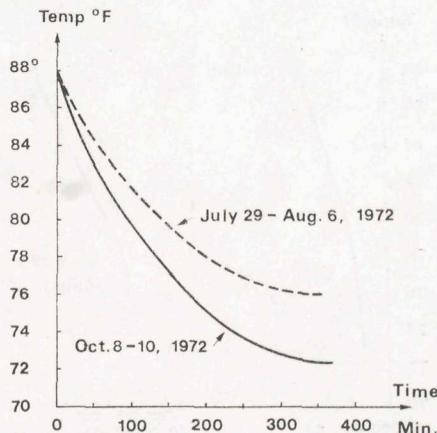
Fig. 5. Decay curve (cooling) for Worden Master gravimeter No. 779.
