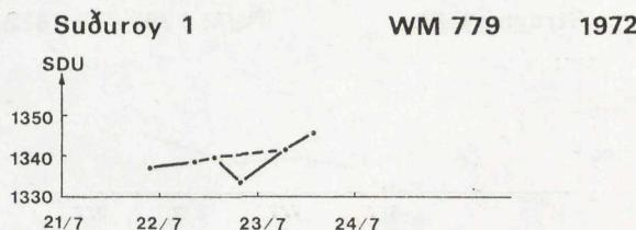
Fig. 4. Drift curve for Worden Master gravimeter No. 779 at station Suðuroy 1.
