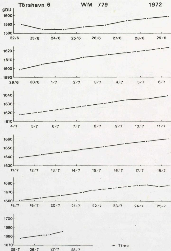
Fig. 2. Drift curve for Worden Master gravimeter No. 779 at station Tórshavn 6; the mean value is 0.27 mGal/day.
