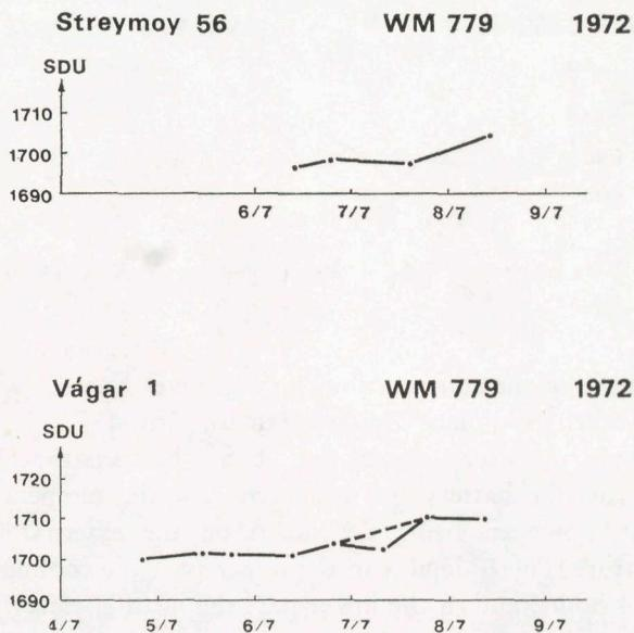
Fig. 3. Drift curve for Worden Master gravimeter No. 779 at station Streymoy 56 and Vágur 1.
