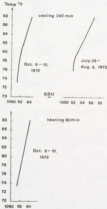
Fig. 6. Cooling and heating of Worden Master gravimeter No. 779.
